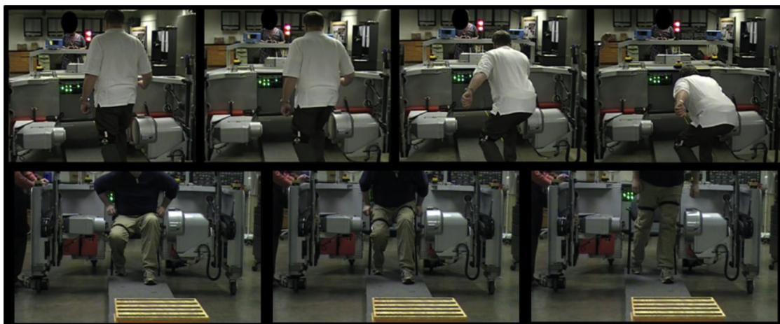
Fig. 1. Subjects performing a deep knee bend (DKB) (top), chair rise (bottom), while under fluoroscopic surveillance with the mobile fluoroscopic unit.
